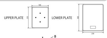
Step 1: Use tapping screws(B) to connect the stand and the upper and lower plates together.
